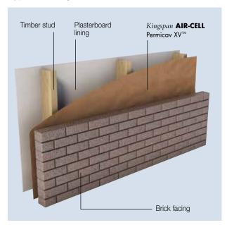
Figure 3 Brick veneer wall installation
